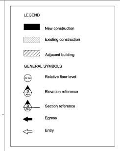
Do not scale this drawing. Figured dimensions only are to be used in preference to small scale drawings. All dimensions are to be checked on site before any work proceeds. Any errors or omissions are to be reported to the designer. If in doubt ask.
